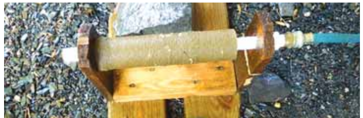
Perforated pvc pipe goes all the way through filter and is connected to a garden hose that's capped shut at the far end.
