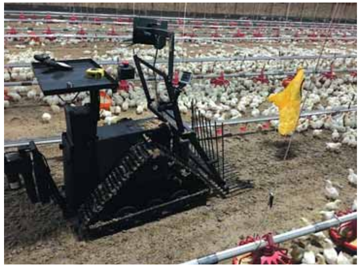
Tracked robot uses a tined loader to pick up dead birds and drop them in a tray for later dumping.
