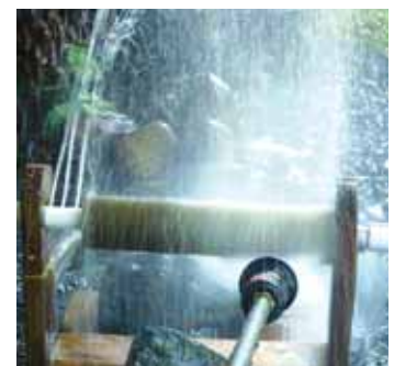
High pressure water just touches bottom of filter, causing it to spin. Centrifugal force cleans filter from the inside out.
