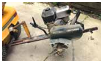
He modified a Craftsman 24-in. walk-behind rototiller to fit the hitch.
