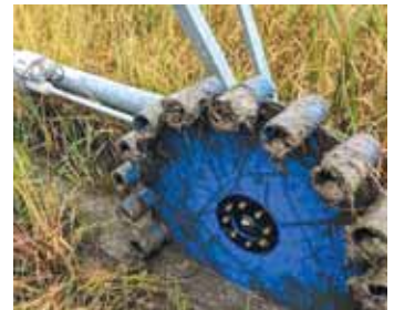
Mud flows through pipes welded to wheel perimeter and falls back into track as pivot moves forward, preventing deep ruts in field. A steel reinforcing ring reduces stress on hub.
