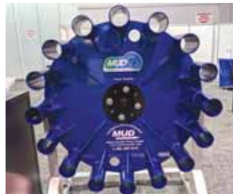
Mud flows through pipes welded to wheel perimeter and falls back into track as pivot moves forward, preventing deep ruts in field. A steel reinforcing ring reduces stress on hub.
