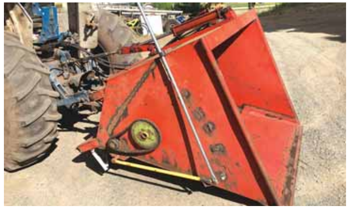
Hydraulic cylinder attached to top link on spreader's 3-pt. hitch allows hopper to tilt back and scoop up material.
