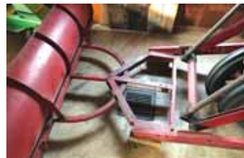
Loader can also be fitted with an angled blade that Stemann welded to a semi-circular frame. It pins onto another frame that bolts onto loader arms.
