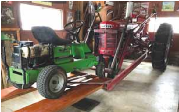
Two 5-ft. long boards, attached between loader arms, make it easy for Stemann to work on riding mowers.
