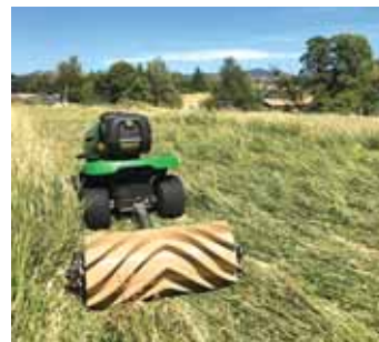
His 3-ft. wide crimper is designed to be pulled by a garden tractor.
