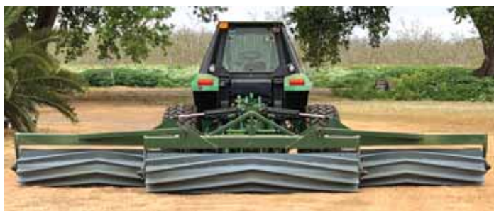
Unruh needed a crimper to turn 8 to 11-ft. tall mustard plants into mulch in his walnut orchard, so he built this 3-pt. mounted, 3-roller model.
