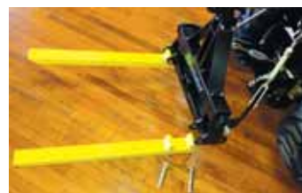
Earth & Turf's 3-pt. pallet fork attachment comes with removable, foldable fork tines, and doubles as a log hitch and receiver hitch.
