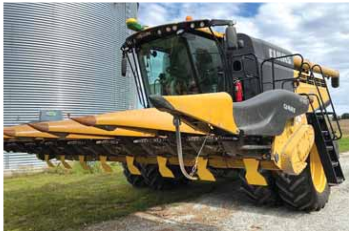
Stalk Knockers set at a 20-degree angle, hovering about 3 1/2 in. above the ground and bending stalks forward away from combine tires.
