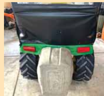
Garden tractor-mounted weight was made by filling an 18-gal. Rubbermaid plastic tub with concrete.
