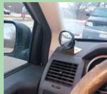
Blind spot mirror is attached to a metal bracket that sticks onto dash.
