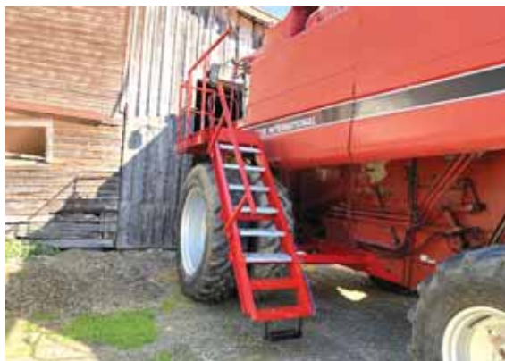
Paul Stermer replaced the rickety ladder on his combine with heavy-duty stairs.
