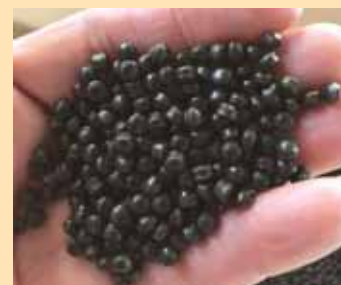
Recycled twine is chopped up, washed, and pelletized for use in other products.
