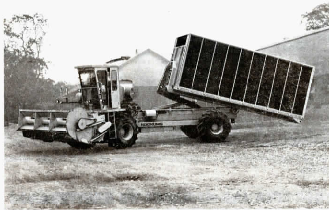
Harvester uses a roll-in, roll-out system to pick up and put down containers. Quick-Attach header can be replaced with windrow pick-up.
