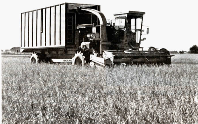
Articulated Kockums 10-ton Whole Crop Harvester is equipped with a 238 hp Detroit diesel, hydrostatic transmission and 4-wheel drive.
