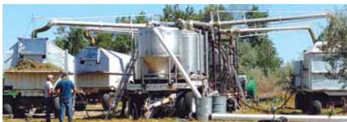
Peppermint is chopped and blown into sealed wagons. Steam is injected into them to produce mint vapor, which is piped to a processor that separates the oil from water. Oil is then siphoned off into 55-gal. drums.
