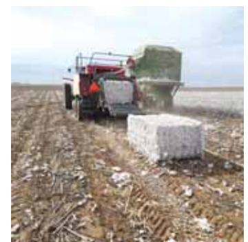
Big square baler is used to bale cotton directly off the stripper, saving time and money compared to using Deere’s $700,000 stripper-baler.
