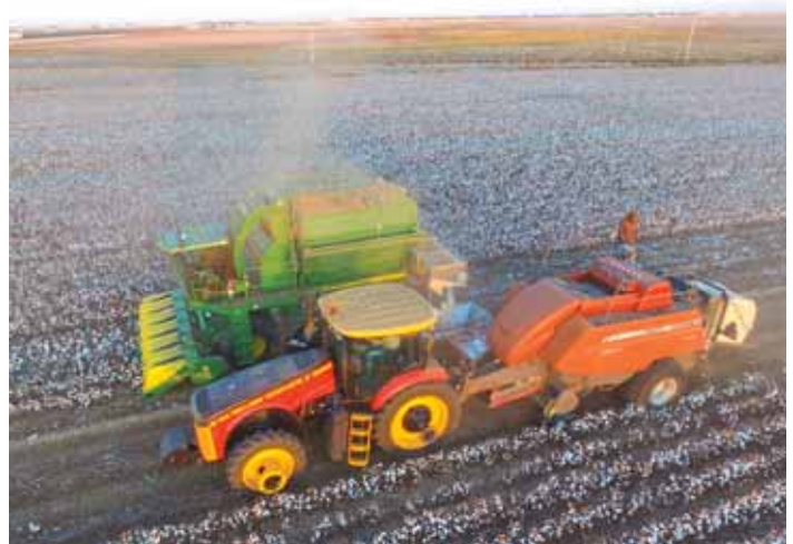
Big square baler is used to bale cotton directly off the stripper, saving time and money compared to using Deere’s $700,000 stripper-baler.
