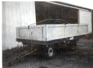
In transport, sides on the float fold up into a portable box.
