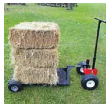
The 2-wheeled Thunderbolt can be used with log tongs to haul more logs, or with a wheeled platform to haul small bales.
