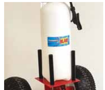
Plow blade works great to push feed to cows in free stalls. Photo at right shows how 4 adjustable metal pillars can be used to hold a spray tank.
