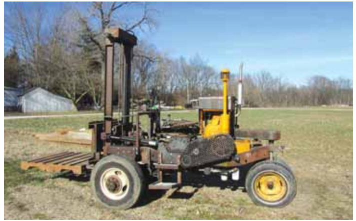
He started with the rear end and frame of a 1970's Chevy 1-ton dually pickup, turning the frame backward so the rear axle and wheels are up front.
