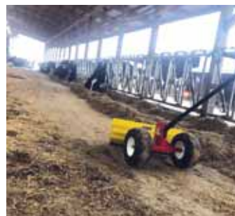
Plow blade works great to push feed to cows in free stalls. Photo at right shows how 4 adjustable metal pillars can be used to hold a spray tank.
