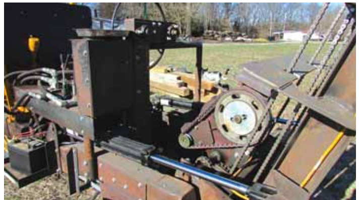
The motor and gearbox off a David Bradley walk-behind tractor is used to chain-drive the forks up or down.
