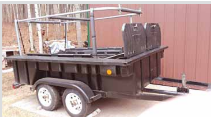
Trailer was made by mounting an old pickup body insert with tool compartments to an angle iron frame and tongue.
