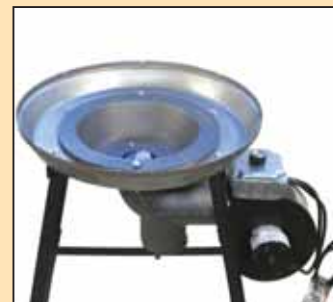
Centaur forges vary from stationary large models with 12 by 14-in. firepots to small 12-in. round models that are easy to move around. Photos show company's Rivet Forge (above) and Handy Forge.
