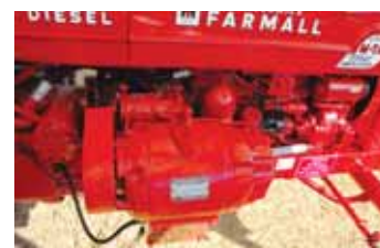
Electrall generators were introduced in 1954, when some rural areas still didn't have reliable electricity. Olson installed one on his Super M-TA tractor (above) that powers his "electric" McCormick 55W baler.
