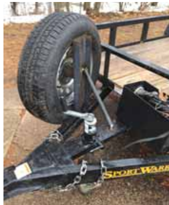
Tire is installed by sliding it over a short horizontal pipe with a pair of matching slots cut into it, then dropping a small steel wedge through both slots and inserting a padlock.
