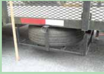
Tire rides in steel cage welded to the trailer frame. Flip-up latch on rack pins onto a tab welded to side of trailer.
