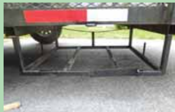
Tire rides in steel cage welded to the trailer frame. Flip-up latch on rack pins onto a tab welded to side of trailer.
