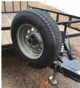
Tire is installed by sliding it over a short horizontal pipe with a pair of matching slots cut into it, then dropping a small steel wedge through both slots and inserting a padlock.
