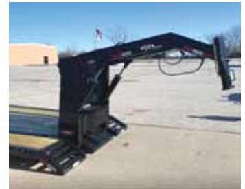
Trailer's gooseneck hitch releases front of trailer bed onto the ground for loading and unloading. The tow vehicle then drives away with gooseneck hitch attached.
