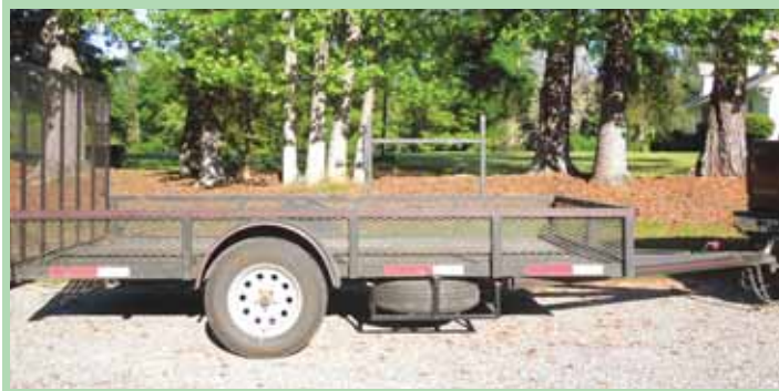
Spare tire carrier mounts under trailer without taking up space on the bed.
