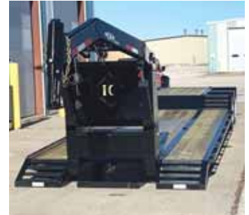
Trailer's gooseneck hitch releases front of trailer bed onto the ground for loading and unloading. The tow vehicle then drives away with gooseneck hitch attached.
