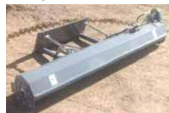
Litter Tiller tills and levels bedding while also releasing moisture and ammonia.
