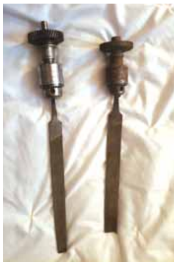
File tang inserted into old drill chuck provides a bigger handle to hold onto. Photo shows 3/8 and 1/4-in. chucks.
