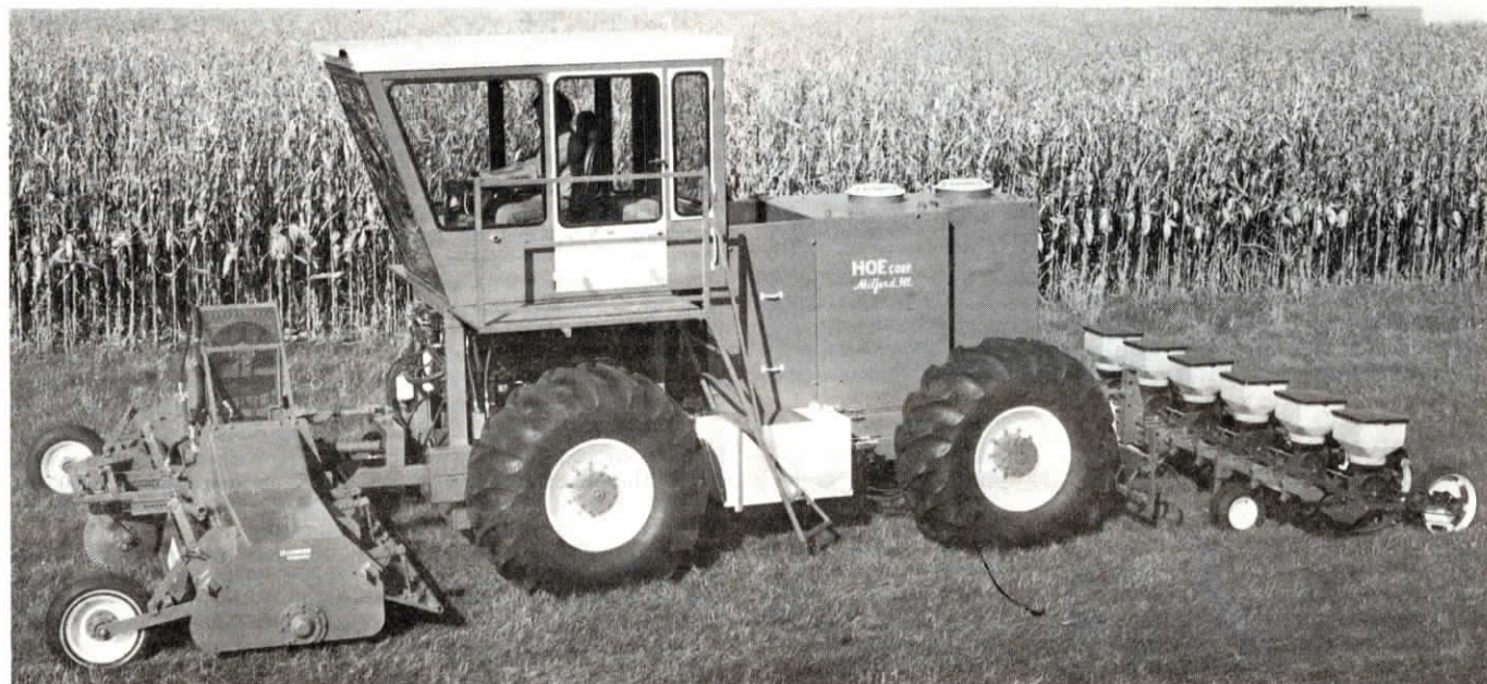
Photo shows, on left, where Tiller-Planter has gone into untouched corn stalks to prepare seedbed, apply fertilizer and herbicides, and plant, all in one operation. Tiller-planter stands in front of same field ready for harvest. The Crows are experimenting to see if chiseling corn stalks in the fall would be desirable.
