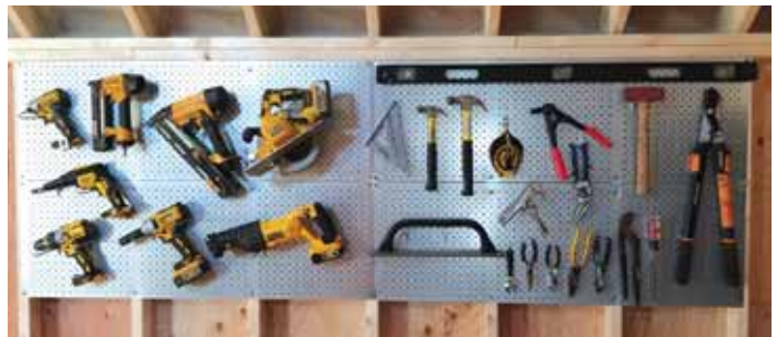
Designed for unfinished shed and garage walls, galvanized steel pegboard is sturdy enough to hang heavy tools.
