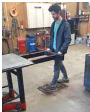
Rolling work bench rides on 4 caster wheels that are lowered to the floor with a foot-operated jack. The table can be quickly lengthened to work on longer objects by pulling out an extension at one end.
