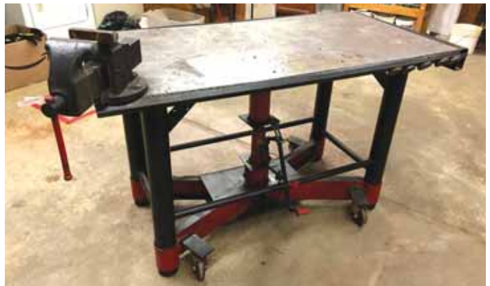
Rolling work bench rides on 4 caster wheels that are lowered to the floor with a foot-operated jack. The table can be quickly lengthened to work on longer objects by pulling out an extension at one end.
