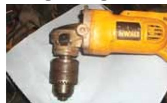
By tapping the back side of an old drill press chuck, Toppen can use his DeWalt cordless angle grinder as a right angle drill.
