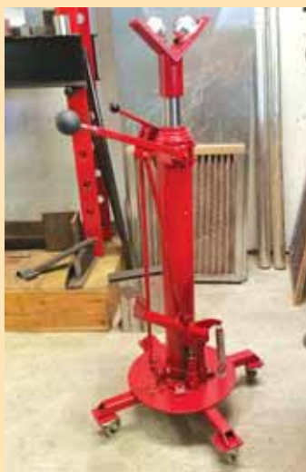
Hydraulic jack is equipped with a 22-in. long cylinder, an internal pump, and a pair of load-bearing transfer balls at the top.
