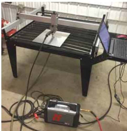
Plasma table comes with user-friendly software, making it simple to operate. Quick torch disconnect (below) allows table to be used with a handheld torch.
