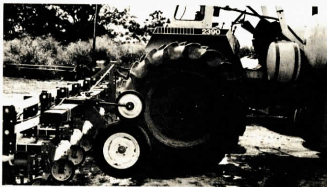
Toolbar-mounted drive wheel, lower center, helps monitor injection system. Note chemical injection line on rear side of cab, upper right.
