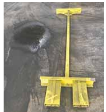
This forklift-mounted, 8-ft. long extender fork is used at the factory to push pallets loaded with 2,000-lb. steel coils toward the front of a trailer.
