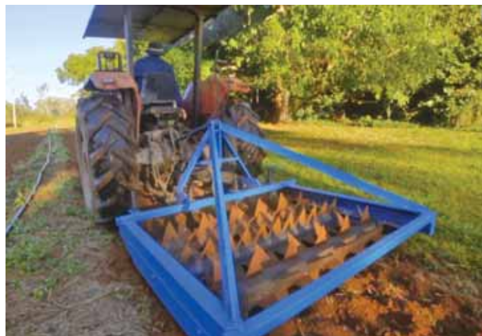
Prongs on front of Rollavator loosen the soil surface, followed by intersecting triangle-shaped tines on steel rollers which leave a fine seedbed.
