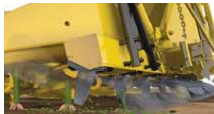
Stalkbuster header option is available on CNH's new rotary corn header. A specially shaped "buster" flail breaks up each row of stubble individually to destroy the overwintering habitat of European corn borers.
