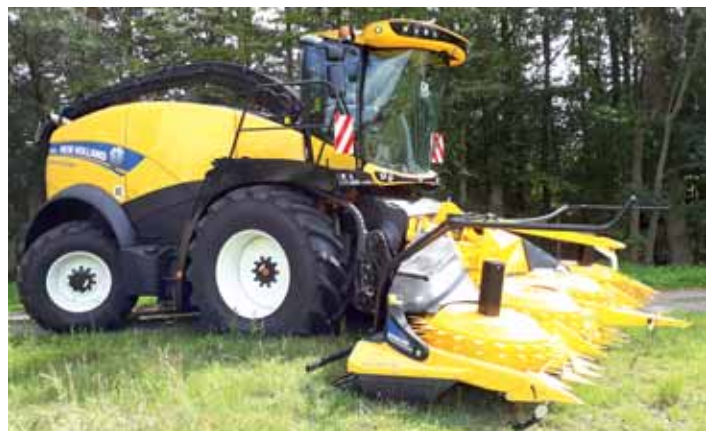
Stalkbuster header option is available on CNH's new rotary corn header. A specially shaped "buster" flail breaks up each row of stubble individually to destroy the overwintering habitat of European corn borers.
