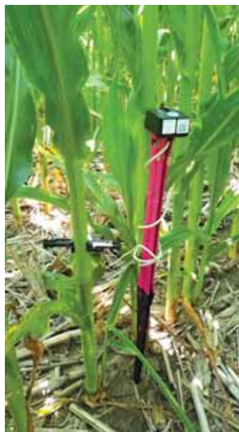
Sensor measures water moving through plant by detecting changes in stalk diameter. The information is analyzed and sent to an app on irrigator's smartphone.
