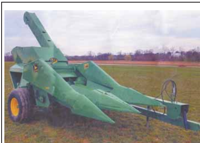
Stoltzfus rebuilt this Deere 300 picker, which he says was the last and best model the company ever made.
