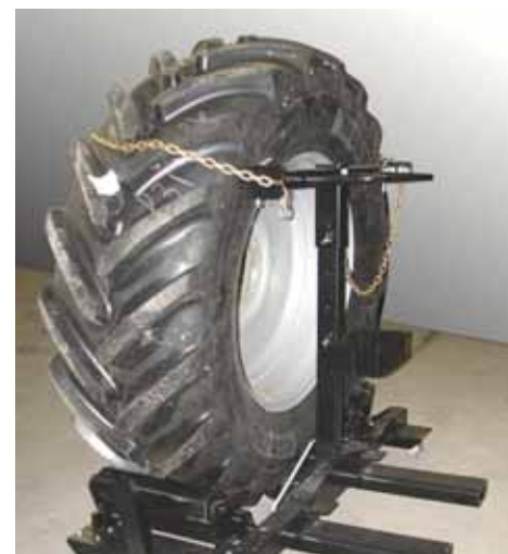
Wheel EZ tire changer comes with a pair of welded-on metal tubes so pallet forks can pick it up. It's built with 2 telescoping halves fitted on each side with 3 metal rollers that support tire.
