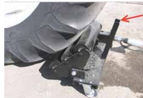
Wheel EZ tire changer comes with a pair of welded-on metal tubes so pallet forks can pick it up. It's built with 2 telescoping halves fitted on each side with 3 metal rollers that support tire.
