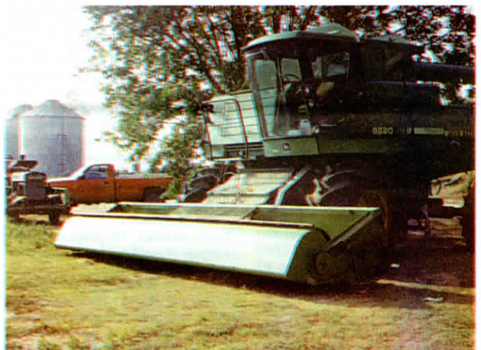
Young fitted the reel (covered by metal shroud) on his stripper combine with "fingers" cut out of durable, and yet flexible, UHMW plastic. The fingers form a keyhole shape that strips grain off stalks.
