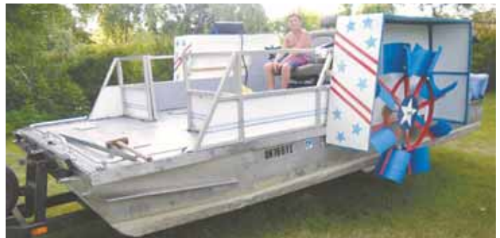
Roy Phlipot's new pontoon boat is driven by a pair of 4-ft. dia. paddle wheels, which are powered by an electric mobility scooter bolted to the deck.
