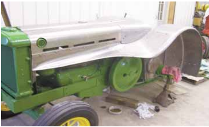
Tractor restorer Scott Hart used an English wheel to form new OEM-style fenders on this John Deere AOS, whose fenders had rusted out.
