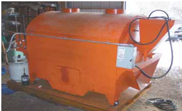
Peanut Roaster repurposed as a second kiln.
