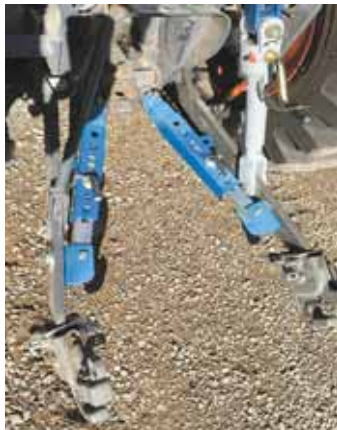
Clockwise from upper left: a length of 5-in. square tubing serves as a chainsaw and splitting wedge holder; chainsaw and splitting wedge in place; chain hooks and receiver hitch welded to loader bucket; modified stabilizers for 3-pt. lower lift arms.
