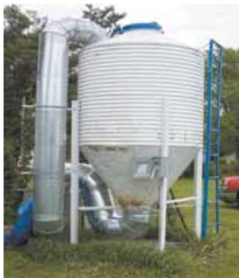
Kiln made from a bulk feed bin.
