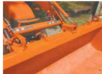
Clockwise from upper left: a length of 5-in. square tubing serves as a chainsaw and splitting wedge holder; chainsaw and splitting wedge in place; chain hooks and receiver hitch welded to loader bucket; modified stabilizers for 3-pt. lower lift arms.
