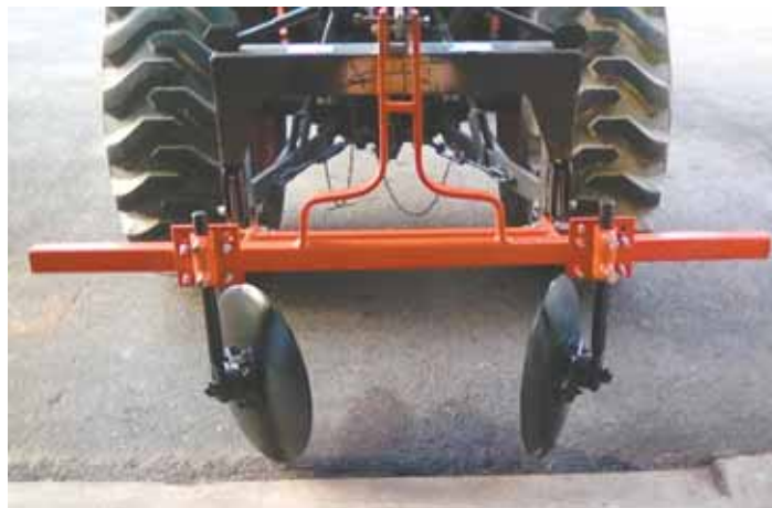
Instead of purchasing a $500 hiller, Robert Weaver built his own for less than $100. He uses it to create beds for his 2-acre garden.
