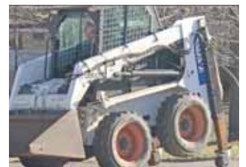
Dual caster wheels at bottom of outriggers let Newnum turn skid loader on a dime, without leaving skid marks on his driveway.
