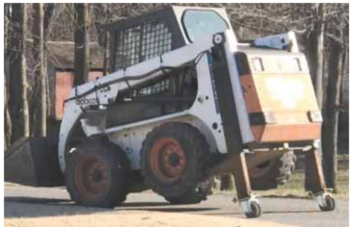
Keith Newnum mounted backhoe outriggers with cylinders on back of his skid loader, which raises the rear end a few inches off the ground.
