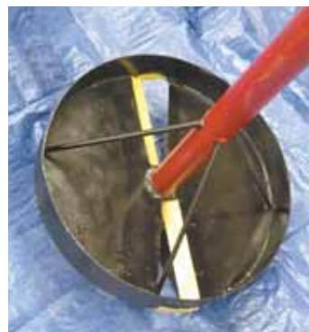
Blades welded to leading edge of slots extend below pan to sweep loose dirt into it.
