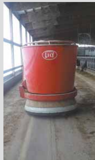
Lely’s robotic feeder takes care of the Malms’ dairy cows and heifers around the clock with almost no human input.
