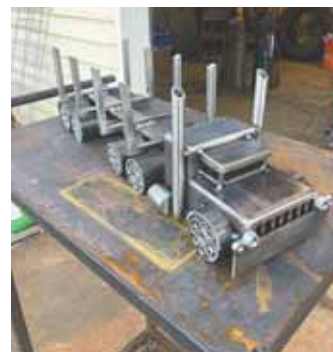
Toy logging truck uses a series of 4-in. tall uprights to hold "logs" in place. The wheels were made by welding nuts together inside cylinders made from round tubing.
