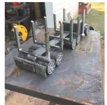
Toy logging truck uses a series of 4-in. tall uprights to hold "logs" in place. The wheels were made by welding nuts together inside cylinders made from round tubing.
