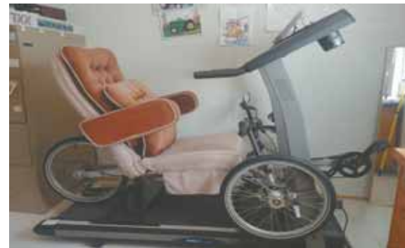
Wilbert Friesen exercises in comfort with a Terra Trike and the reclining seat from an old van. Trike's rear wheel rides on treadmill.
