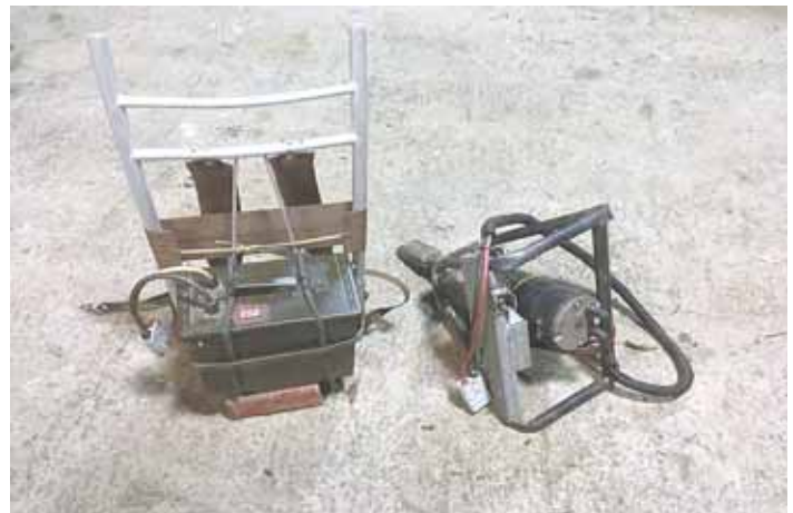
Giant cordless "drill" is made from a forklift steering motor powered by lithium battery packs. Workers use it to install ground anchors on 300-ft. long hot house tunnels.
