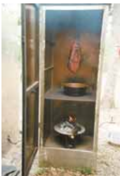
Burner at bottom hooks up to a propane bottle located outside smoker.
