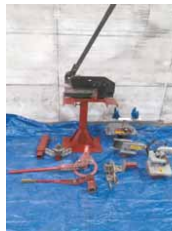
Top section of the tool mount can be removed to position tools closer to the floor for better leverage.
