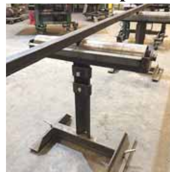
Sand lined up the stands in a straight line, spaced 4 ft. apart, and drops pins through them into holes he drilled in the floor.
