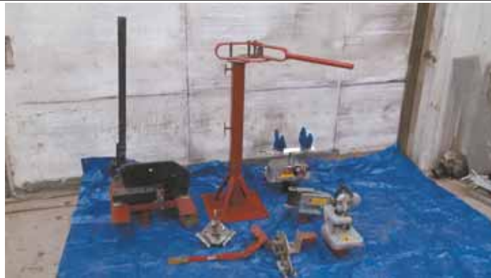
McLaen attached 2-in. hitch tubes to several metal working tools. That lets him quickly insert them into the top of the tool mount.
