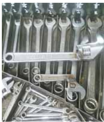
McCulley bought cheap 12 and 6-in. wrenches and then cut off the heads, turned them 90 degrees, and welded them back on.
