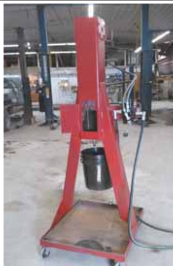
McLaen's hydraulic-operated crusher can handle even large truck and tractor filters. Access door for inserting filters is open, at left. Photo at right shows the crusher components which include crushing chamber, hydraulic cylinder, and square tubing piston.
