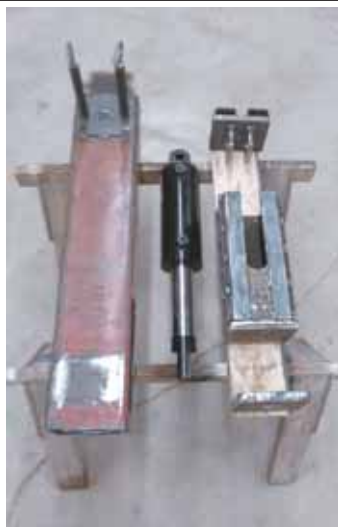
McLaen's hydraulic-operated crusher can handle even large truck and tractor filters. Access door for inserting filters is open, at left. Photo at right shows the crusher components which include crushing chamber, hydraulic cylinder, and square tubing piston.
