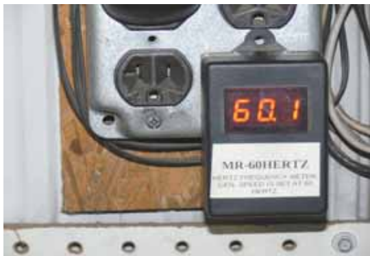
"Hertz meter" plugs into any generator-powered electrical outlet to help protect electrical equipment when running a pto-powered generator.
