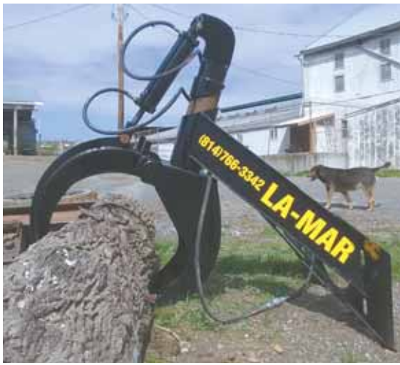
Heavy-duty log grapple quick-tatches to any skid loader and can be swiveled a little more than 180 degrees.
