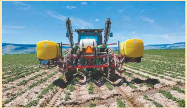
A pair of big spray tanks mount on a 3-pt. platform that rides behind Rathbun's Deere tractor.
