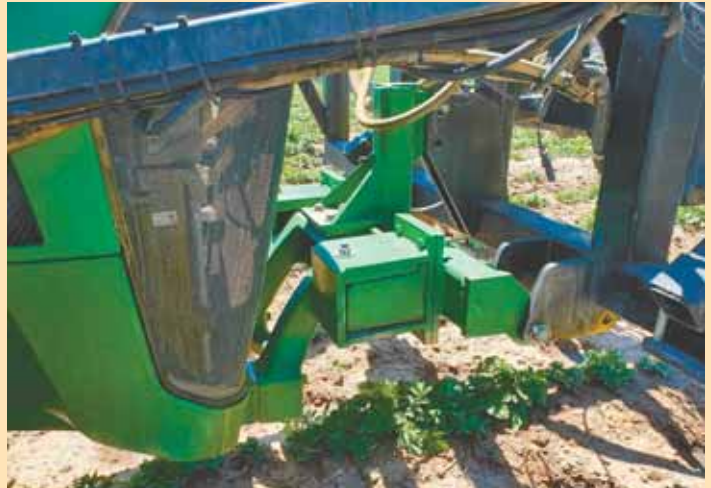
Spray boom mounts on a bracket that holds tractor's front weights.
