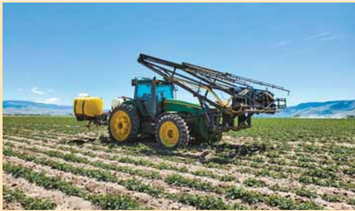
"It lets me spray my fields without looking back," says Phil Rathbun, who converted a 3-pt. mounted sprayer with an 80-ft. boom to a front-mount model.
