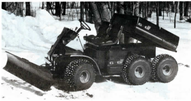
Front hitch can be used to mount 5-ft. mower or this 6-ft. snow plow.
