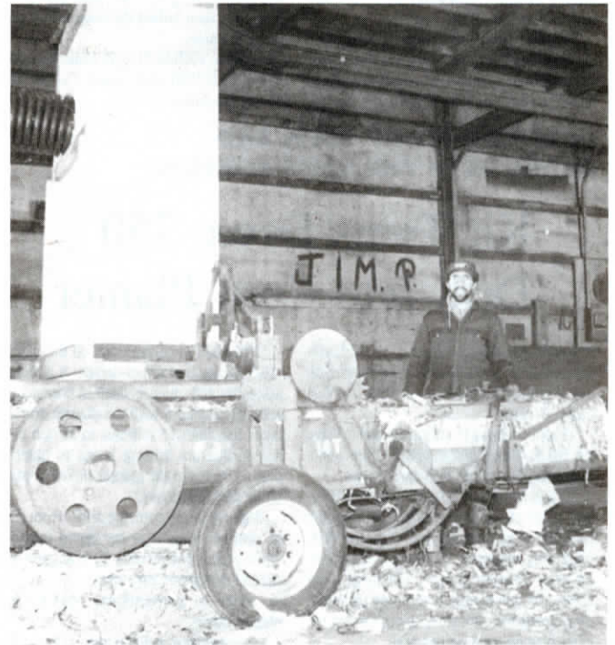
Jaquet modified Deere 14T baler and New Idea Uni-Harvester silage chopper. Chopped paper is blown through piece of 12-in. dia. plastic drain tile into drop box.
