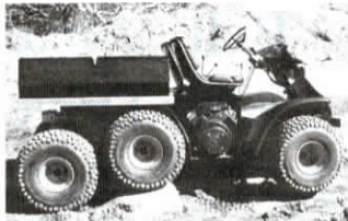
Walking beam rear axles ride up independently over rocks and other obstacles.
