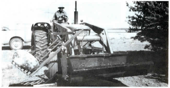
Tined fork digs out rock, then rotates upward until rock slides down into bucket.
