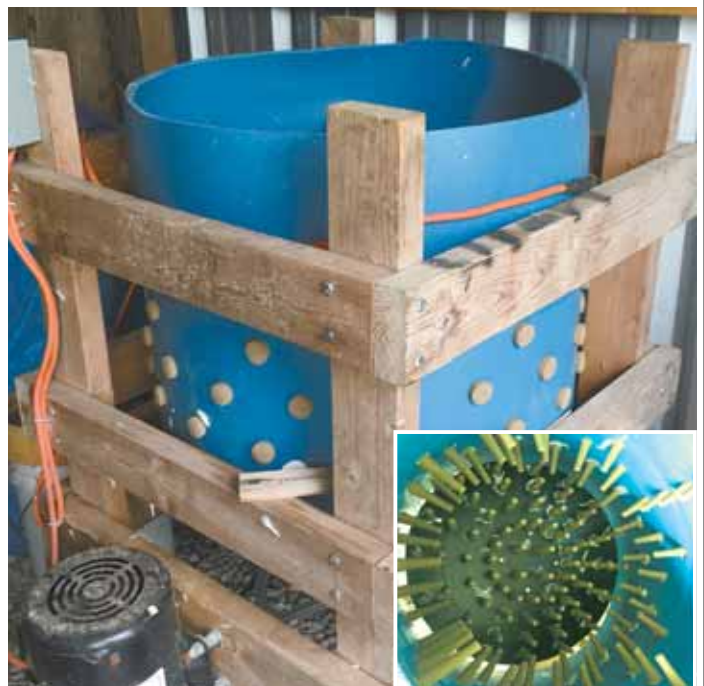
Jimmy Rhea made this chicken plucker out of a plastic 55-gal. drum that sits inside a wooden frame. A 1/2 hp. electric motor belt-drives the drum, which has rubber fingers attached inside.
