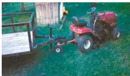
Lightweight trailer dolly was built using parts of an old tricycle, with a ball hitch attached to the seat. Shaw uses dolly to pull a 2-wheeled trailer behind his garden tractor.
