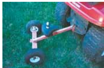
Shaw drilled a hole through the seat, then inserted ball and screwed a nut on underneath.
