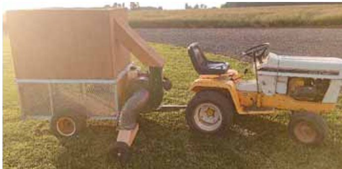
Kuenzi uses his home-built trailer to vacuum grass clippings and leaves behind a Cub Cadet riding mower.
