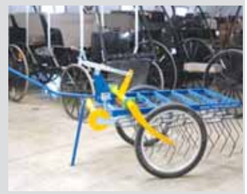
Tension on the tines adjusts hydraulically from the tractor seat. A variety of sizes are available, from a 30-in. wide garden size (below) up to 100-ft. wide field units.
