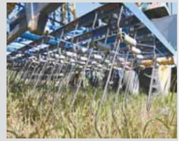
Tension on the tines adjusts hydraulically from the tractor seat. A variety of sizes are available, from a 30-in. wide garden size (below) up to 100-ft. wide field units.
