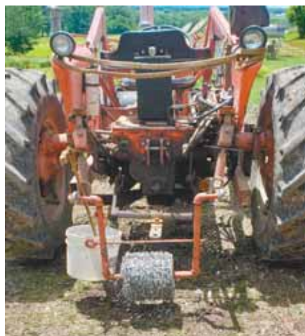
Wire unroller clips onto 3-pt.'s lower lift arms and is fitted with a "safety rod", which keeps the wire from snapping back at the operator.
