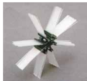
Husk brushes mount in metal brackets that clamp onto the original square shafts on a New Idea corn picker.
