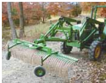
Hewitt adapted a Harbor Freight 3-pt. quick hitch to fit the quick-tach mounting brackets on his loader. He attaches a 3-pt. rock rake to smooth out his driveway.
