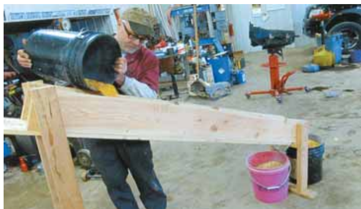
Home-built wooden chute has a 1/2-in. screen that removes any foreign matter in corn.
