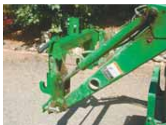
Hewitt adapted a Harbor Freight 3-pt. quick hitch to fit the quick-tach mounting brackets on his loader. He attaches a 3-pt. rock rake to smooth out his driveway.
