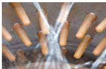
Chicken plucker comes with 110 replaceable rubber fingers mounted inside a stainless steel tub. A built-in irrigation ring supplies water to help remove feathers from birds.
