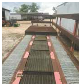
Trailer is equipped with 2 draglines, allowing Simmonds to quickly unload small square bales off the back end. Metal panels cover dragline when trailer is loaded with bales.
