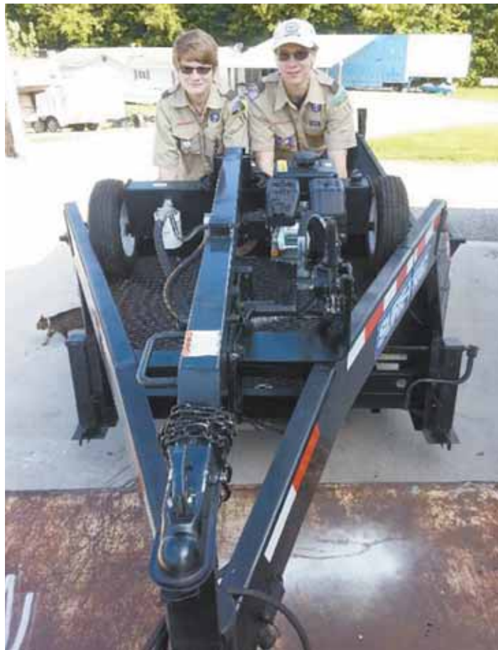
Jadin and Brock Seiler replaced the slow-working electric pump on their gooseneck dump trailer with the power unit off a log splitter.
