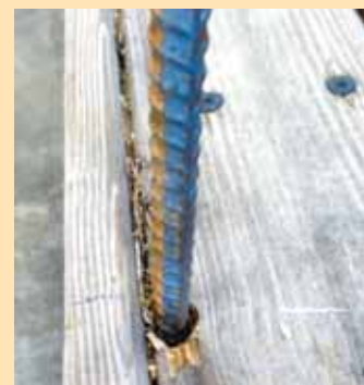
Capen cut 20-ft. lengths of 1/2-in. rod in half and bent them into a hoop shape. He then drilled holes on each side of the wagon floor and pushed the hoops into place.
