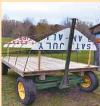
Capen cut 20-ft. lengths of 1/2-in. rod in half and bent them into a hoop shape. He then drilled holes on each side of the wagon floor and pushed the hoops into place.
