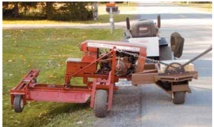
Deck extends from back side of engine and hood. "It works great to mow hard-to-reach areas under trees and out over ditches," says Larry Johnson.
