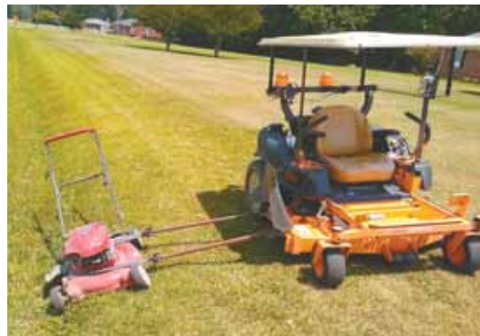
Side-mounted push mower extends 30 in. out to the side of zero-turn mower and swivels on a pair of 30-in. arms made from square tubing. Bolts that run through both ends of the arms serve as hinge points, allowing push mower to flex up or down.
