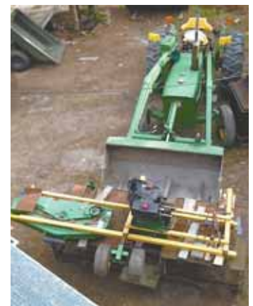
Mower deck is driven by the 12 hp. engine off a walk-behind snowblower. It mounts on a steel frame that pins onto 2 metal tubes bolted to bucket floor.
