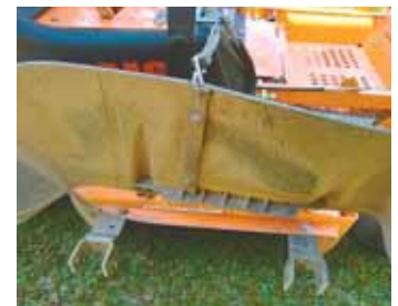
Side-mounted push mower extends 30 in. out to the side of zero-turn mower and swivels on a pair of 30-in. arms made from square tubing. Bolts that run through both ends of the arms serve as hinge points, allowing push mower to flex up or down.
