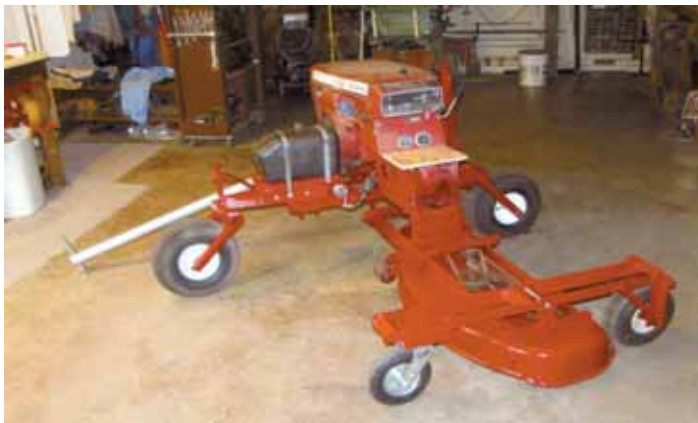
Side-mount mower was built by cutting up a Wheel Horse riding mower. The engine and hood mount sideways on a steel frame fitted with mower's original front wheels.
