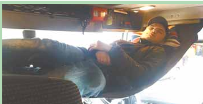
Portable hammock fits across width of truck cab using a sewn-in beads trapped over the tops of both doors.
