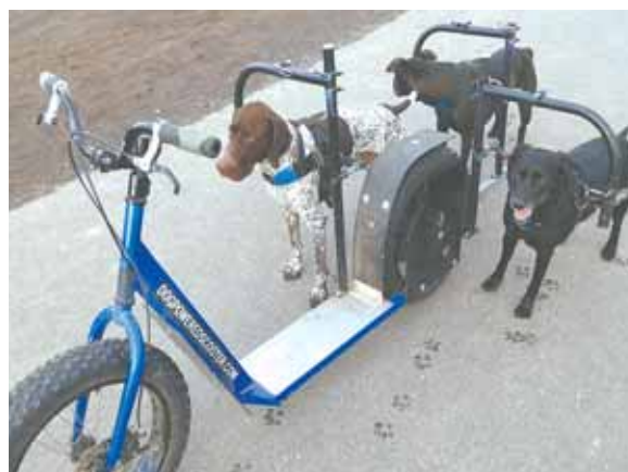
Secured by a 2-point harness, dog pulls from the side and behind the driver. Scooter is narrow enough to run 2 or 3 dogs at a time down sidewalks.
