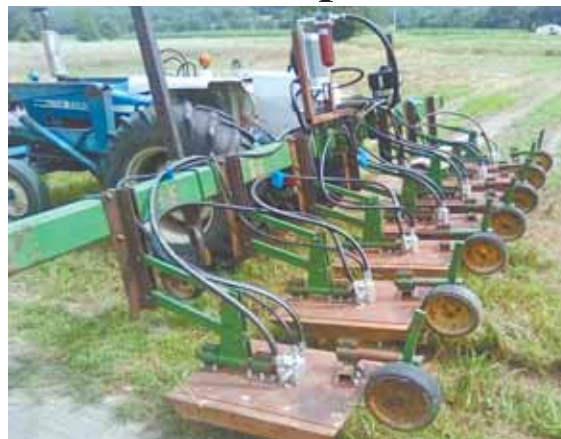
Los's 3-pt. mounted mower clips weeds off between crop rows before they can go to seed. Mowers are operated by a pto-driven hydraulic pump.
