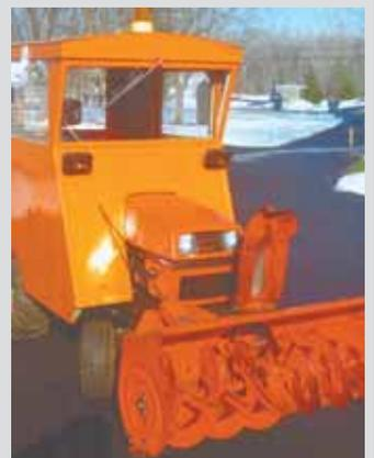
Home-built cab is equipped with a wiper, defroster, 15,000 btu heater, mirrors, flasher, and extra lights. Johnson rebuilt the snowblower.
