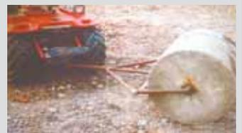
Concrete roller rotates on a small pipe that rides inside a bigger one. Telescoping tongue hooks up to both sides of roller.
