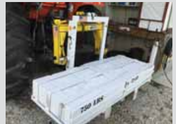
To offset the weight of the Path Slayer, Myers made a 3-pt. mounted, 750-lb. counterweight out of 35-lb. cement blocks.
