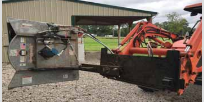
The 44-in. deck on the Path Slayer rotary cutter can be set at 11 different positions.
