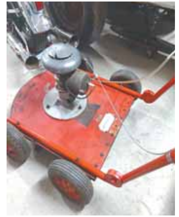
Sensation mower originally came with a wooden deck and wheels, reflecting the lack of metal available during WW II.
