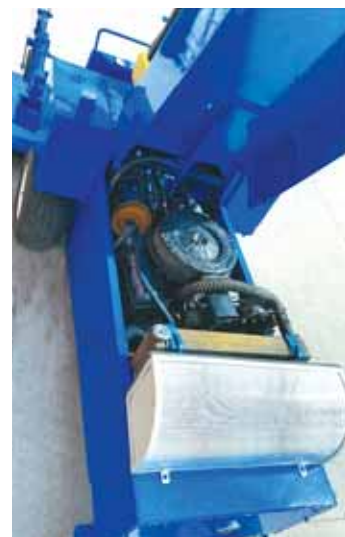
Don Robinett built this riding mower 30 years ago, and now at 88 years old he still uses the machine regularly. It's powered by an all-aluminum Buick V-8 gas engine. The air intake for the radiator was made from an old Massey Harris combine sieve.
