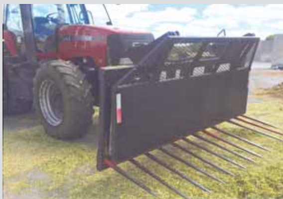
Top of push-off blade is hinged and hydraulically moves forward off a stationary frame to eject haylage from forks.
