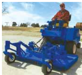
Don Robinett built this riding mower 30 years ago, and now at 88 years old he still uses the machine regularly. It's powered by an all-aluminum Buick V-8 gas engine. The air intake for the radiator was made from an old Massey Harris combine sieve.
